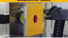
Not only for shielding efficiency and reduction but also for improving image quality with the reduction of scattering, collimators are existing to be used on the detector or the source side.
