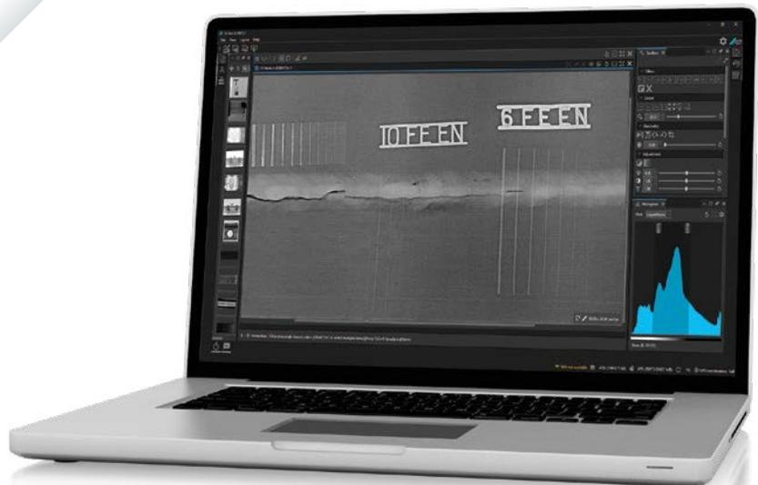
*Computed radiography (CR) is the digital replacement of conventional X-ray film radiography and offers enormous advantages for inspection tasks - the use of consumables is virtually eliminated and the time to produce an image is drastically shorter.*
