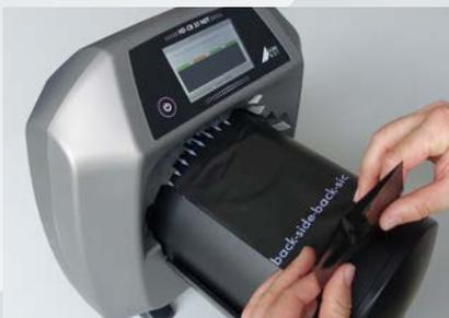
**4** Feed in the imaging plate - intake then starts automatically.
