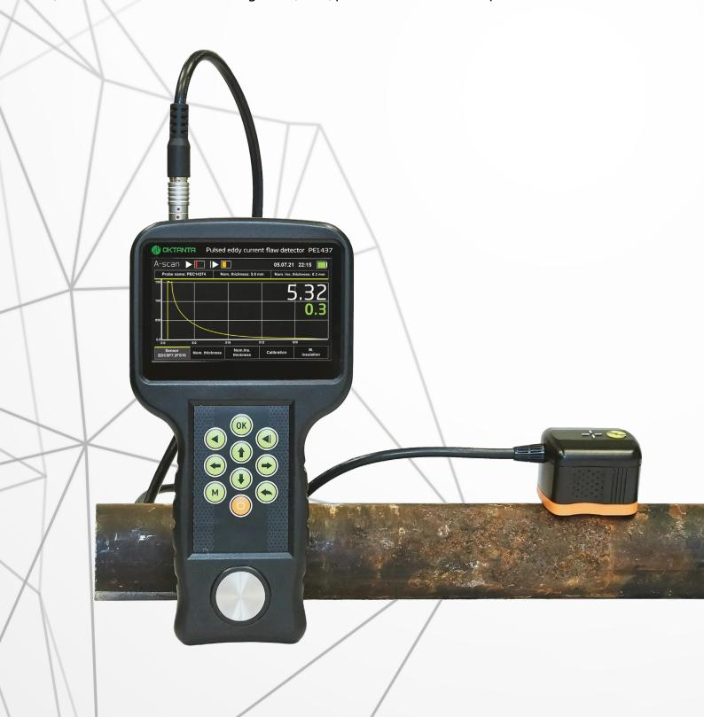
PE1437 can detect corrosion areas in steel objects without any preparation of surface. There is no need to remove scale, dirt, paint, etc. The total thickness of scale deposits or paint can be up to 30 mm.
