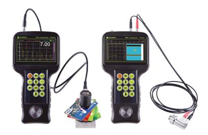
EM1401 is easily and quickly calibrated using specified thickness or sound velocity, as well as measured metal type. The mode of working with strobes allows using the gauge as a flaw detector with direct entry. A high working speed of the device (32 measurments per second) allows you to measure the thickness of long objects easily and quickly.
