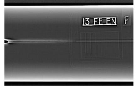
Thin-walled stainless steel cylinder with longitudinal weld seam.
